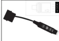
C) If your motherboard doesn't have any RGB lighting system, plug the RGB hub adapter into the internal RGB controller in the way showed in the picture above. Then connect the Internal RGB controller to a PSU connector.
