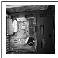
Install M/B / Instala la placa base.
