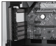
Remove PCI slots.
