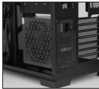
Put power supply (align location).
