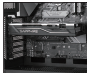
Put VGA (align location).
