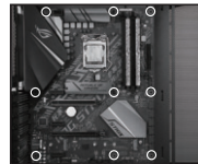
Fix M/B by screws.
