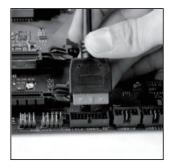
Plug in USB 3.0 connector to the motherboard
