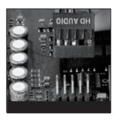
Plug in the AUDIO HD connector to the motherboard.
