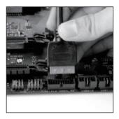
Plug in the USB 3.0 connector to the motherboard.
