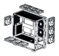
**TOP:** Support 3\*120 mm / 2\*140 mm Support 240/280/360 mm Liquid cooler
