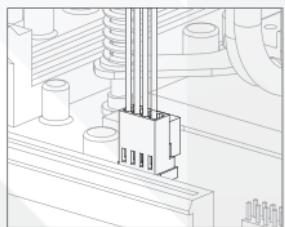
Connect CPU small 4pin power cable to "CPU\_FAN" header on the motherboard.
