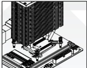
3) Put the heatsink onto the CPU, tightening the bracket screws into the backplate to secure the heatsink firmly.
