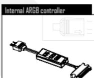
B) If your motherboard doesn't have any ARGB lighting system, plug the ARGB Hub adapter into the internal ARGB controller in the way showed in the picture above. Then connect the Internal RGB controller to a PS4 connector.
