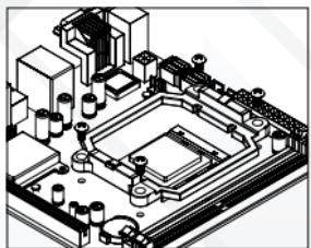
1) Remove original AMD plastic retention frame, but keep the backplate.
