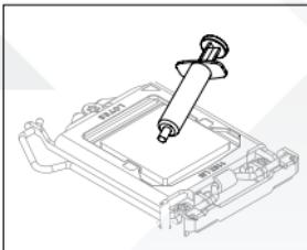
2) Apply a thin layer of thermal grease to the CPU surface.
